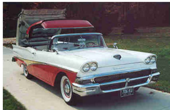
30. A 1958 Ford Fairlane transitioning from hardtop to convertible.
